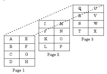
MATLAB internally represents the data for this three-dimensional array in the following order:
