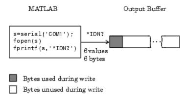
The \*IDN? command consists of six values because the terminator is automatically written. Moreover, the default data format for the fprintf function specifies that one value corresponds to one byte. For more information about bytes and values, see "Bytes Versus Values" on page 16-10. fprintf and the terminator are discussed in "Writing Text Data" on page 16-32.
