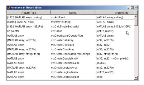
The types used in the argument lists and return values are MATLAB types, not C types. For more information on types, see "C and MATLAB Equivalent Types" on page 3-18.
